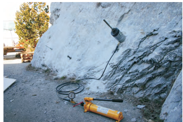
Offset in rock anchor shell with anchor rod
